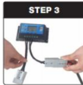
Then connect the controller onto the battery.
