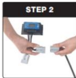
Disconnect the controller and battery.
