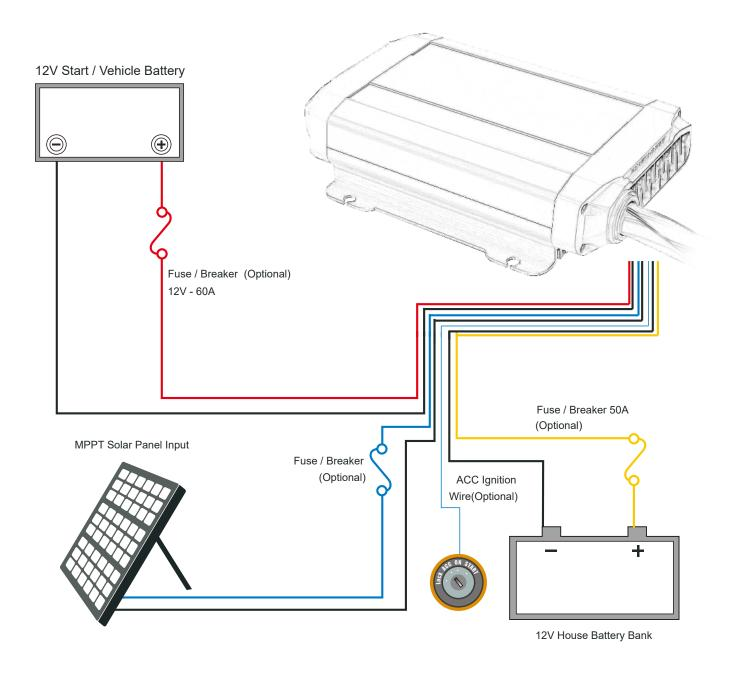
**NOTE:** First connect the ACC line to the ignition of your vehicle. Then turn your key to the ACC position when engine starts, which will be detected by the DC-DC charger. And your auxiliary battery will be charged via the main battery.
