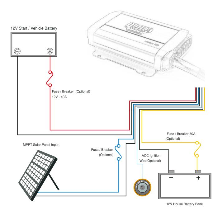
**NOTE:** First connect the ACC line to the ignition of your vehicle. Then turn your key to the ACC position when engine starts, which will be detected by the DC-DC charger. And your auxiliary battery will be charged via the main battery.
